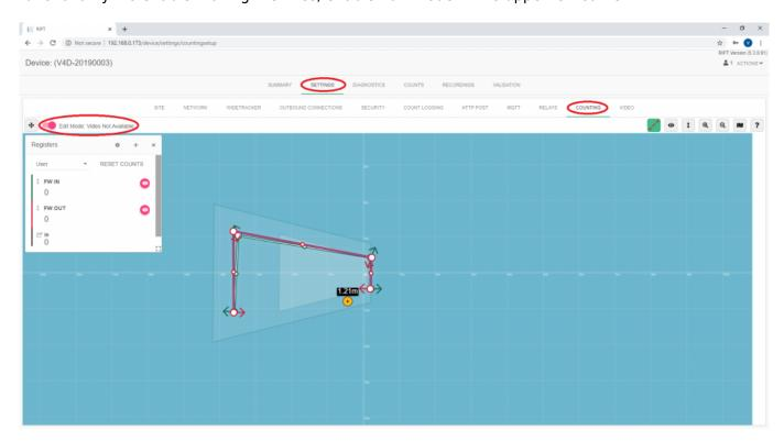
Configure the count lines so that people are counted accurately. When positioning the lines, always ensure that there is enough 'initialisation' space for the counter to recognise a person and start tracking them – lines should be positioned away from the edge of the field of view.
