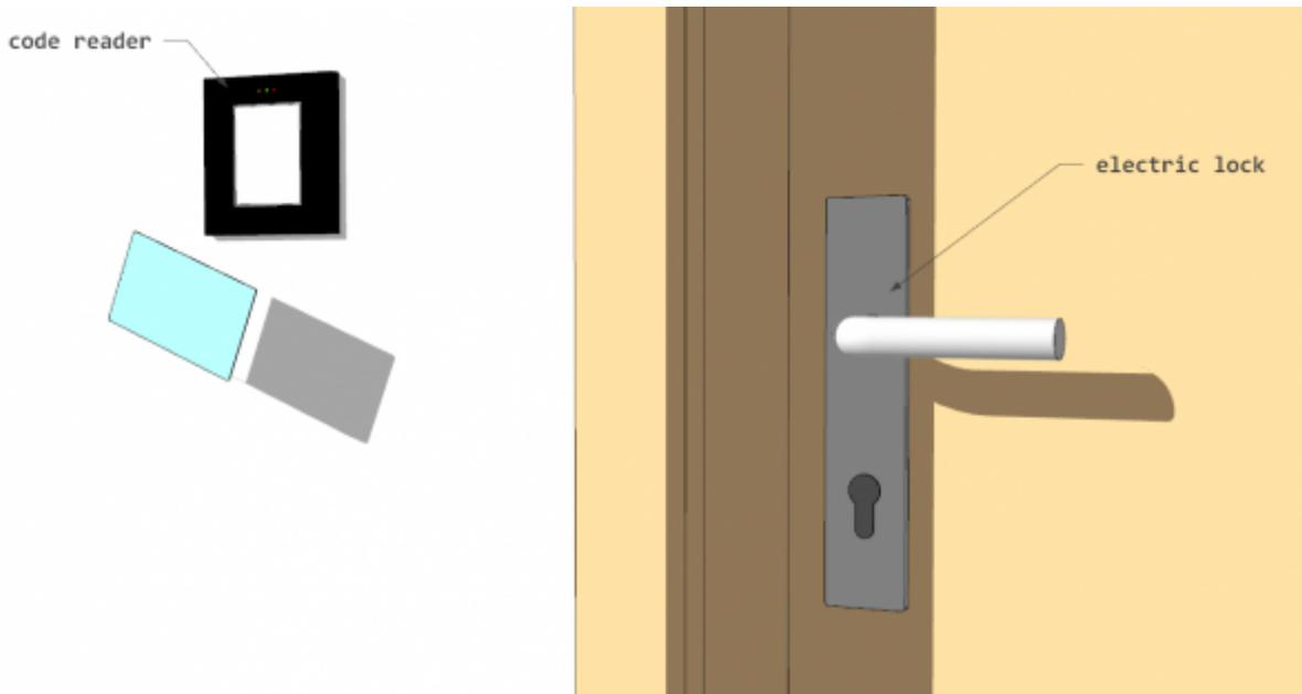
Both are connected to an **access controller** that can operate independently, in conjunction with other controllers in local network, or in conjunction with an **advanced access control application** which can be installed on a local server or as a cloud service on **HIQ Universe**.
