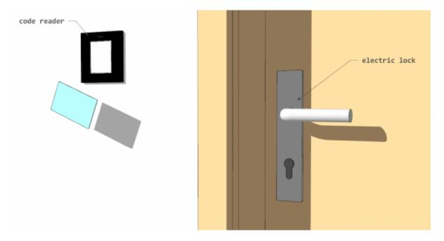
Both are connected to an **access controller** that can operate independently, in conjunction with other controllers in local network, or in conjunction with an **advanced access control application** which can be installed on a local server or as a cloud service on **HIQ Universe**.
