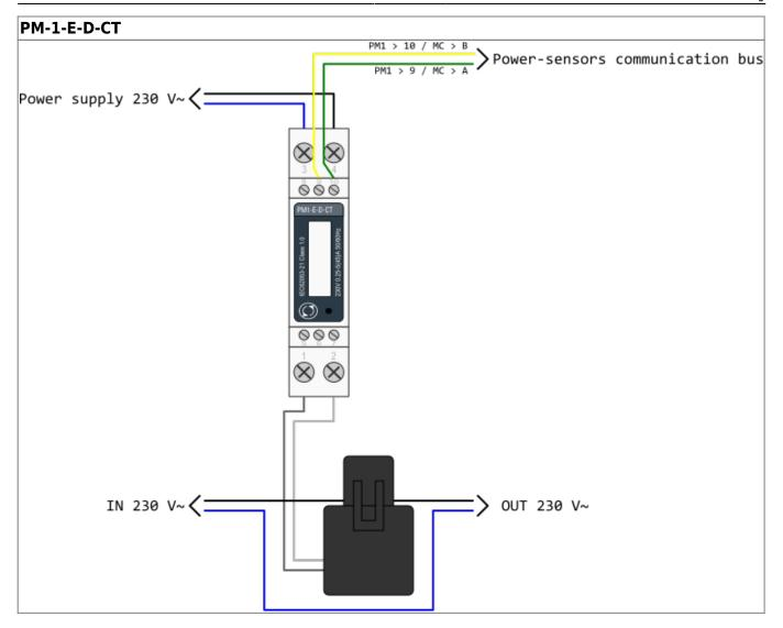
Example of HEMS G2 wiring diagram:
