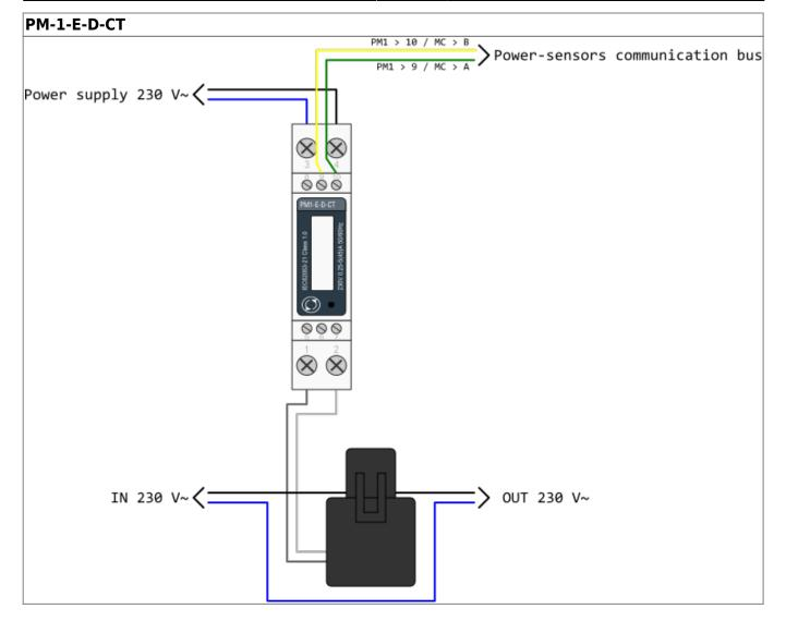
Example of HEMS G2 wiring diagram:
