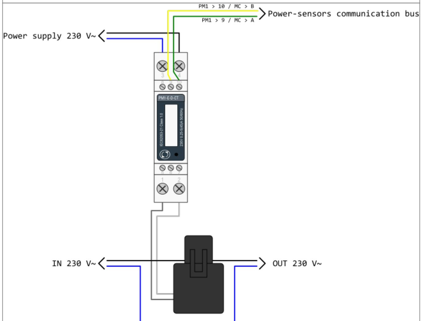
Example of HEMS G2 wiring diagram:
