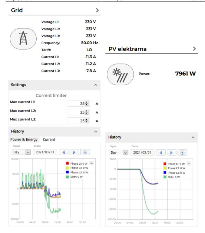
Producers present devices or systems that produce electrical energy. Example of such devices are solar power plant, wind power plant, diesel generator and others. An example on the following figure shows solar power plant.
