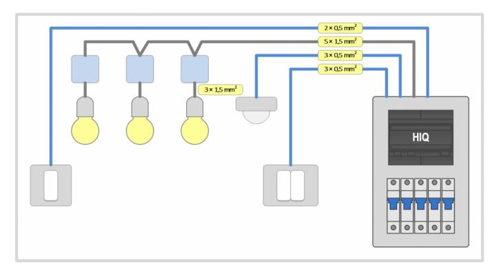
All light ballasts are wired to DALI bus with an appropriate wire gauge (usually  $5 \times 1.5 \text{ mm}^2$ )
