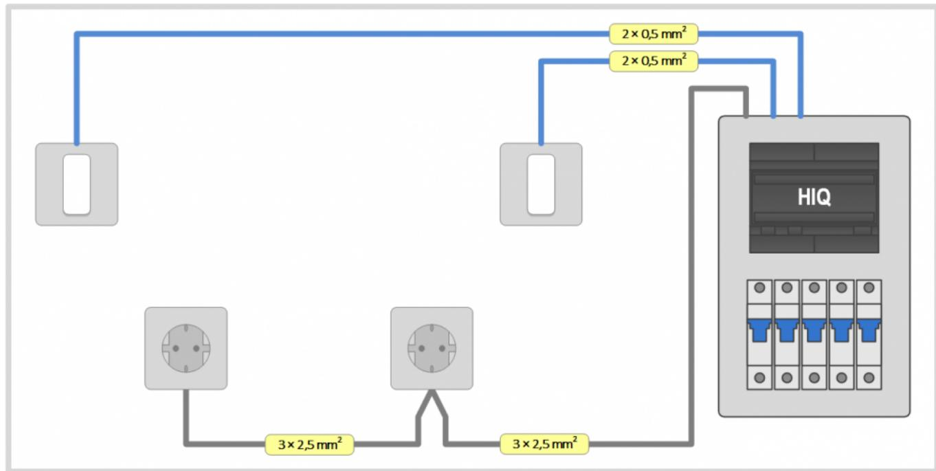
Sockets group is wired to the distribution box with an appropriate wire gauge (usually  $3 \times 2,5 \text{ mm}^2$ )
