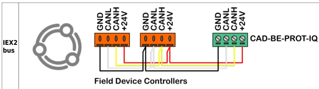
All field modules are connected to the IEX bus with  $2 \times 2 \times 0,8 \text{ mm}^2$  cable.
