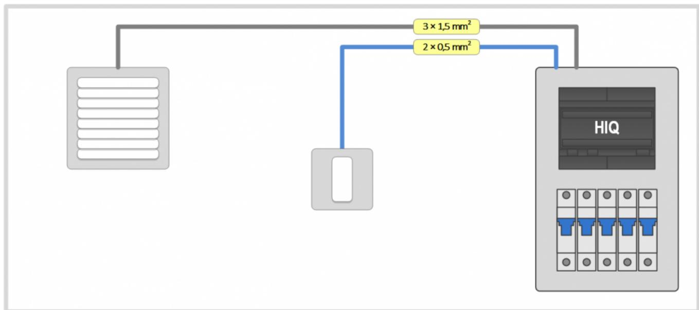
Exhaust fans are wired directly to the distribution box with an appropriate wire gauge (usually  $3 \times 1,5 \text{ mm}^2$ )
