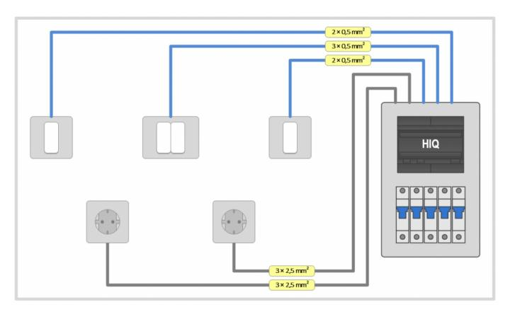
Individual sockets are wired directly to the distribution box with an appropriate wire gauge (usually  $3 \times 2.5 \text{ mm}^2$ )
