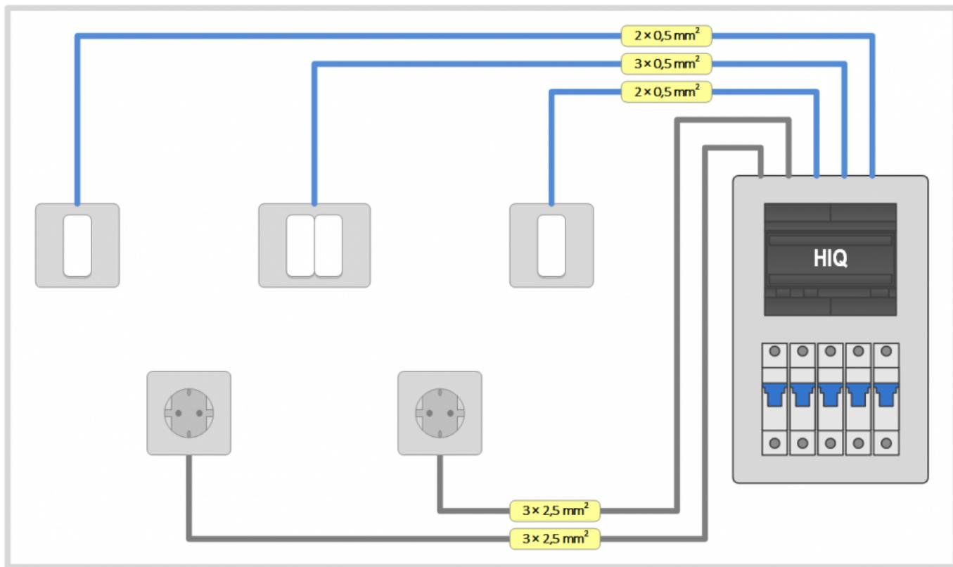
Individual sockets are wired directly to the distribution box with an appropriate wire gauge (usually 3 x 2,5 mm<sup>2</sup>)
