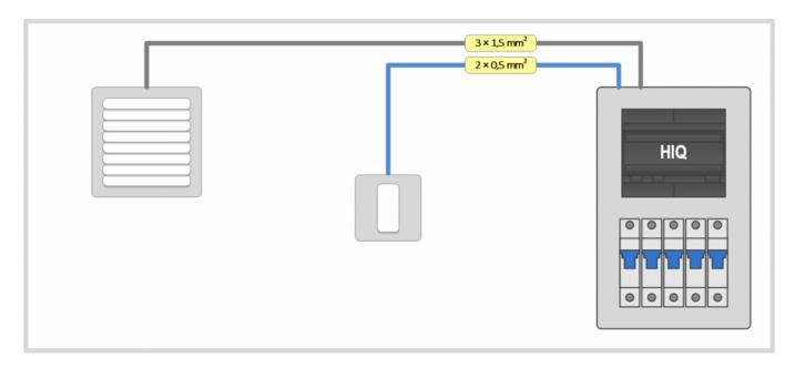
Exhaust fans are wired directly to the distribution box with an appropriate wire gauge (usually  $3 \times 1.5$  mm<sup>2</sup>)
