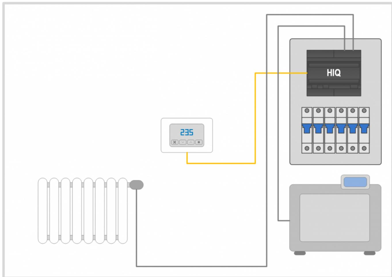
Radiator valves and boiler enable signal are wired directly to the distribution box with an appropriate wire gauge (usually  $3 \times 1,5 \text{ mm}^2$ )
