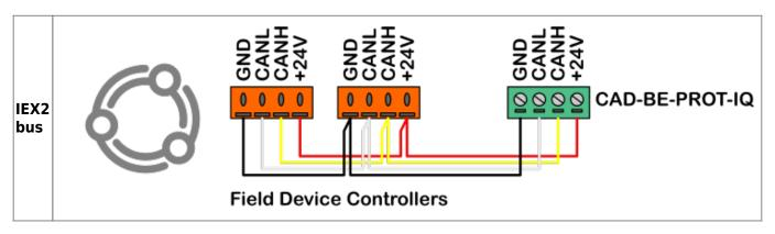
All field modules are connected to the IEX bus with  $2 \times 2 \times 0.8 \text{ mm}^2$  cable.
