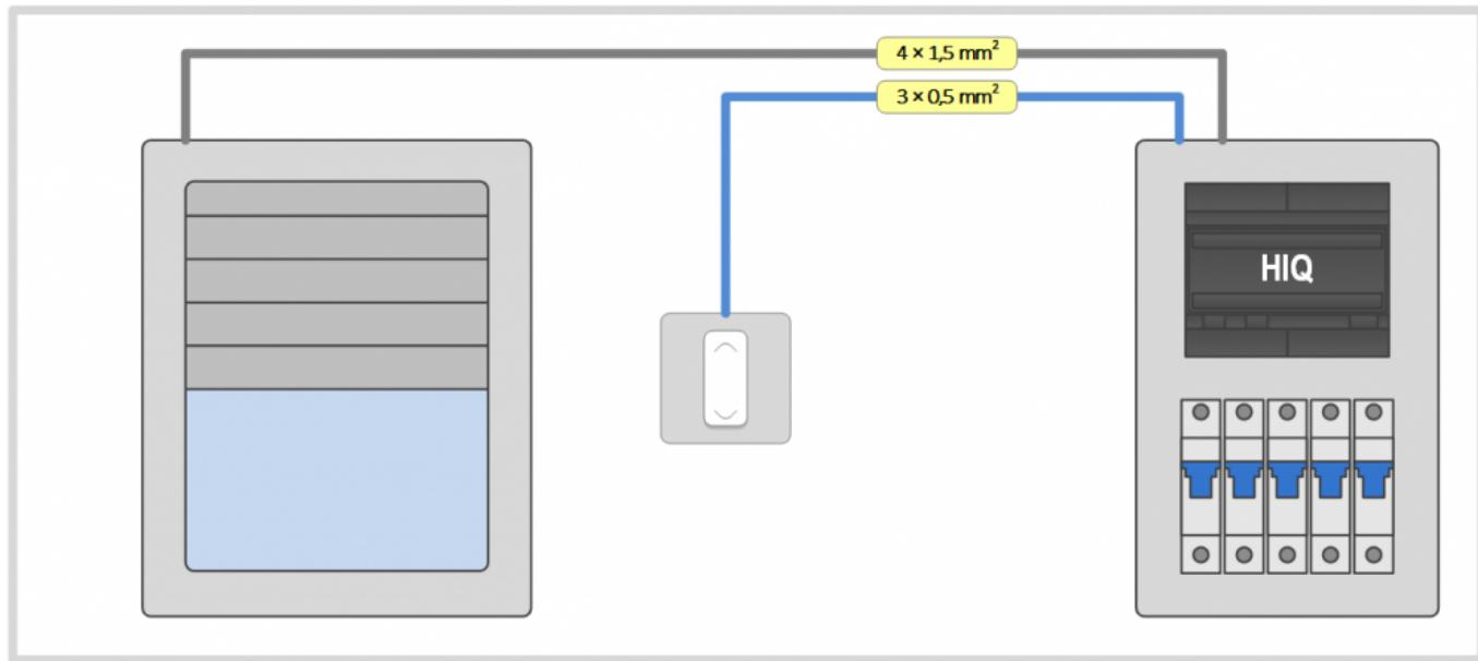
Blind motors are wired directly to the distribution box with an appropriate wire gauge (usually  $4 \times 1,5 \text{ mm}^2$ )
