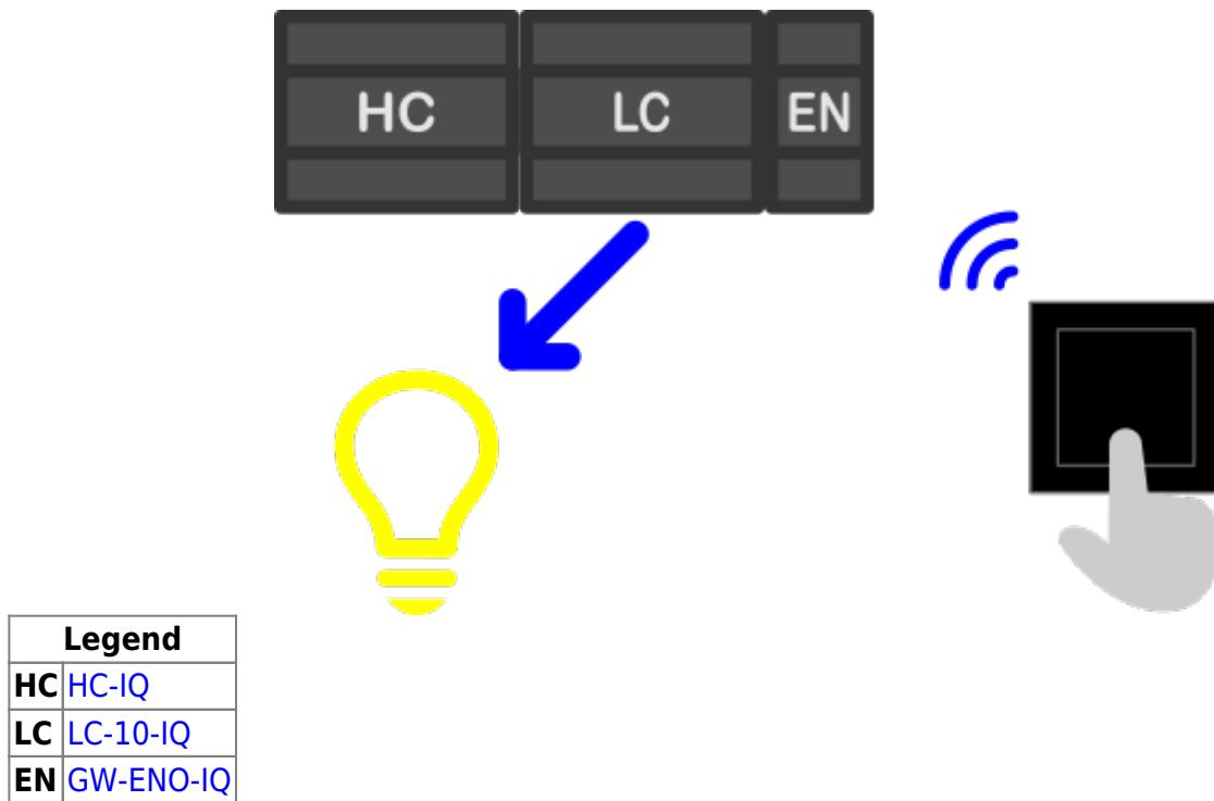
Following example show how to toggle light and / or scene with EnOcean wireless batteries-less push-button.
