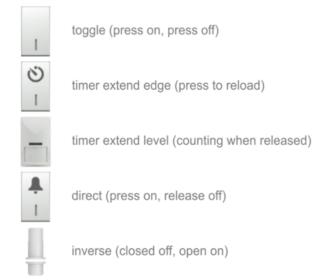
Input mode defines how input affect the output. Basic functions are handled internally by light controller, night mode and ready light are handled with master controller.
