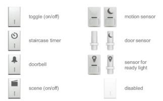
Input mode defines how an input controls the output. Toggle, staircase, doorbell, motion and door sensor are handled internally. Scene and ready light are handled by master controller.
