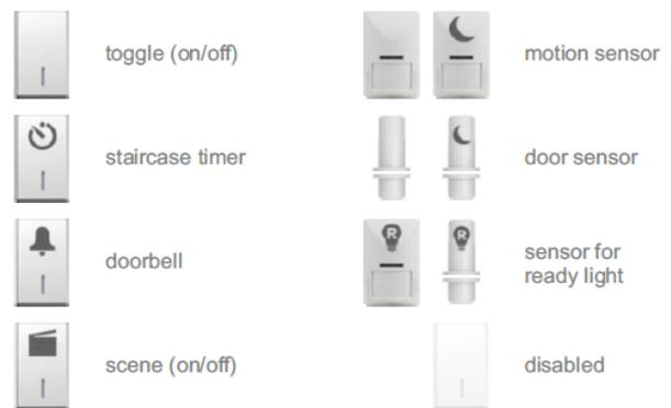
Input mode defines how an input controls the output. Toggle, staircase, doorbell, motion and door sensor are handled internally. Scene and ready light are handled by master controller.
