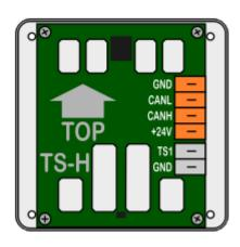
When installing: "Autoaddress" button will link FC-1-IQ unit with lowest serial number with thermostat with lowest serial number and so on.
