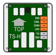
When installing: "Autoaddress" button will link FC-1-IQ unit with lowest serial number with thermostat with lowest serial number and so on.
