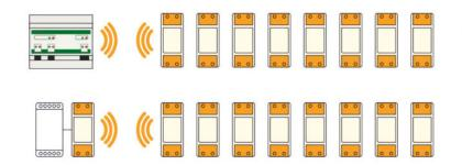
Cybro-3-RFM, acting as modbus master, connected to 8 wireless relays (200..207).
