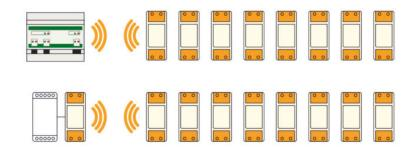
Cybro-3-RFM, acting as modbus master, connected to 8 wireless relays (200..207).
