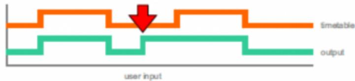
When timetable controls an output, manual override is possible at any time, timetable will catch on with the next transition.
