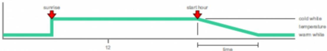
To configure evo light, first experimentally find the best light for early and late evening. Start hour and transition time should be configured so the warm light is reached at least one hour before bedtime.
