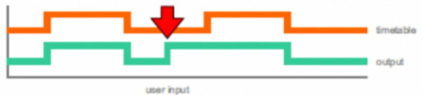
When timetable controls an output, manual override is possible at any time, timetable will catch on with the next transition.
