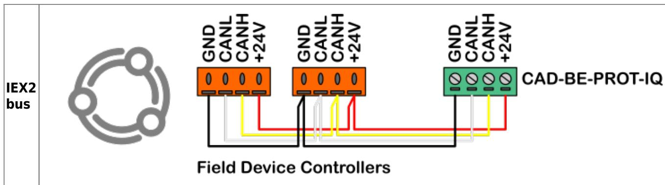
All field modules are connected to the IEX bus with 2 x 2 x 0,8 mm<sup>2</sup> cable.
