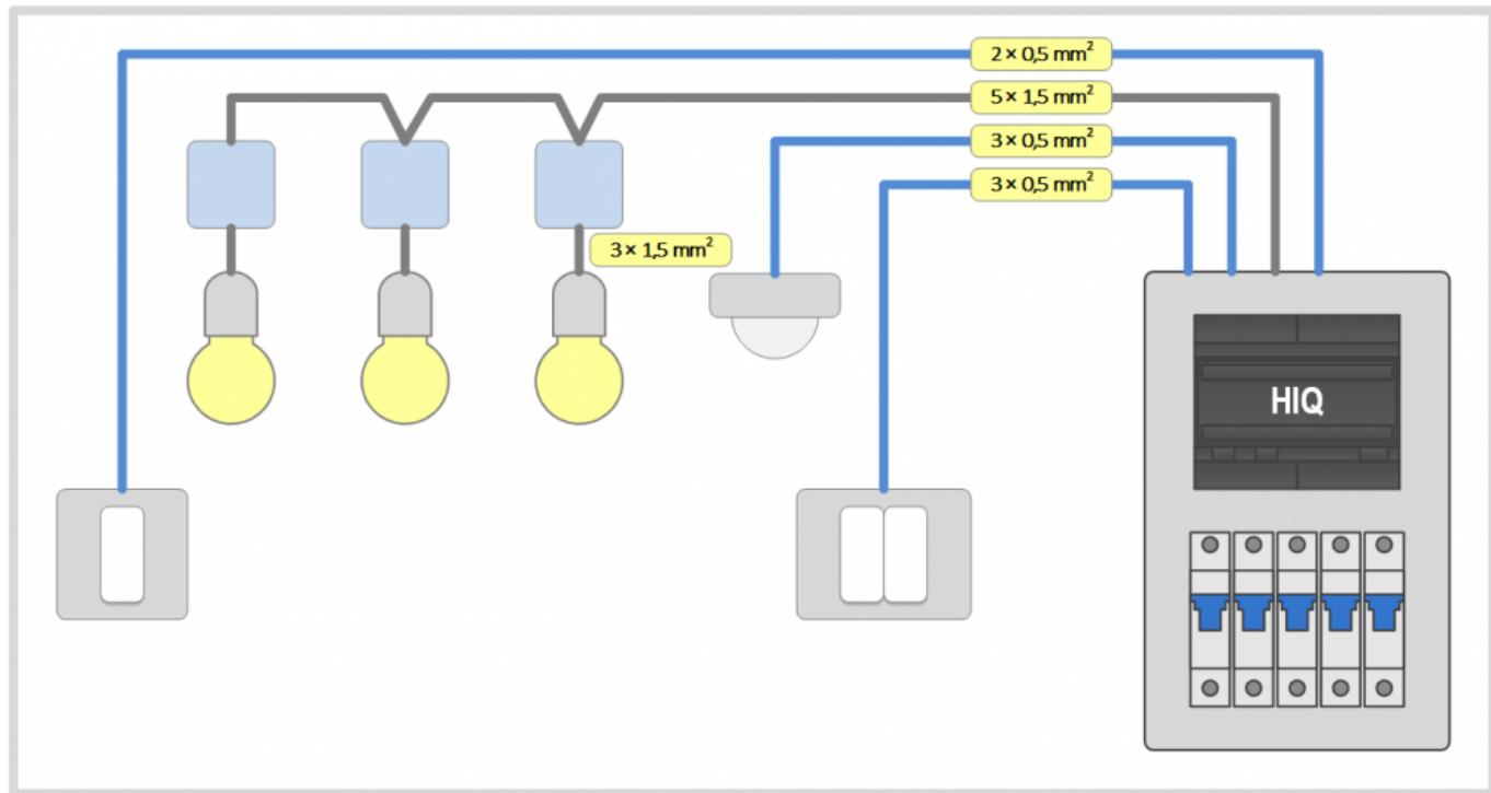
All light ballasts are wired to DALI bus with an appropriate wire gauge (usually  $5 \times 1,5 \text{ mm}^2$ )
