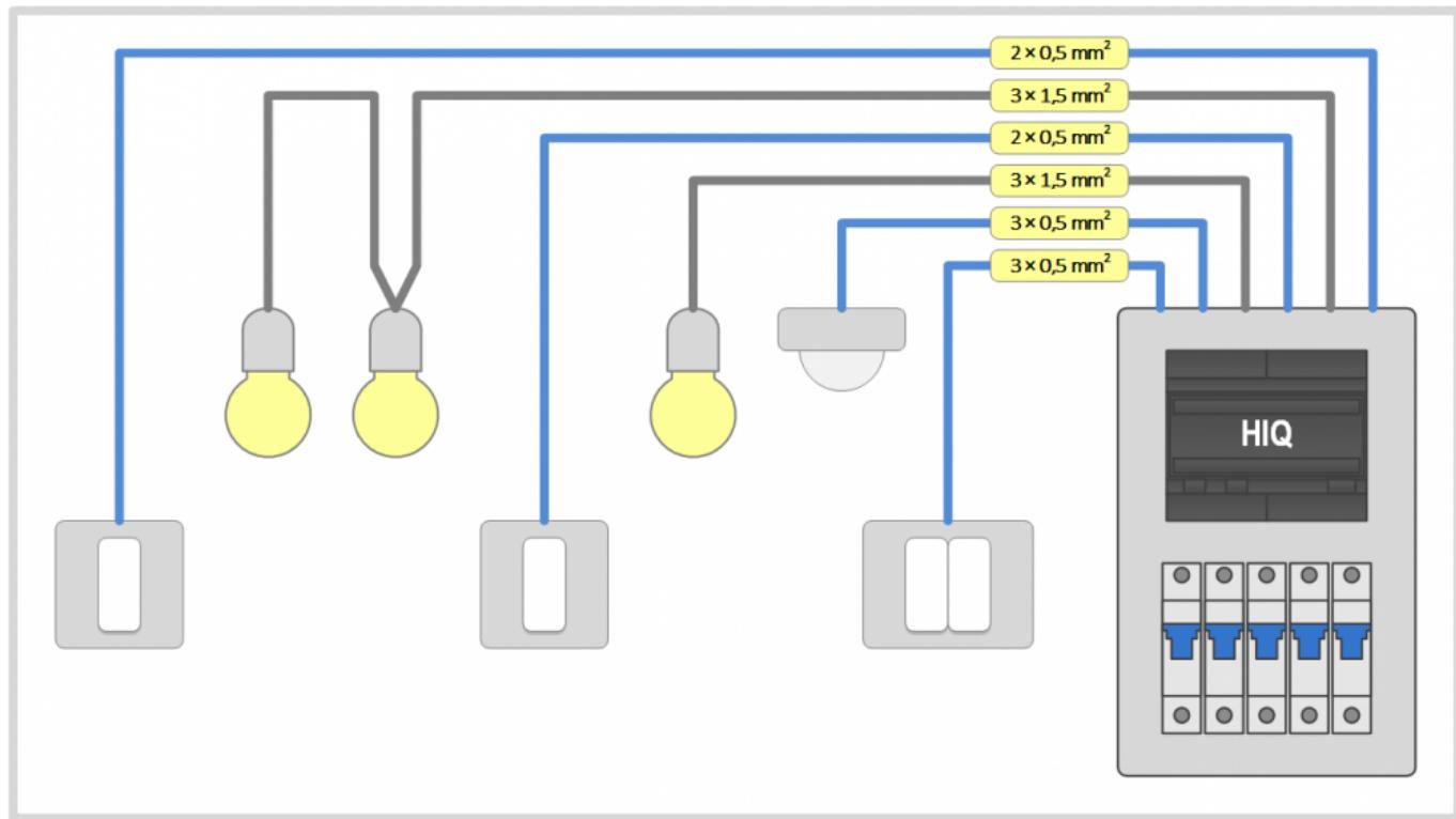
Individual lights (or hard-wired light groups) are wired directly to the distribution box with an appropriate wire gauge (usually  $3 \times 1,5 \text{ mm}^2$ ).
