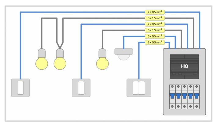
Individual lights (or hard-wired light groups) are wired directly to the distribution box with an appropriate wire gauge (usually  $3 \times 1.5 \text{ mm}^2$ ).
