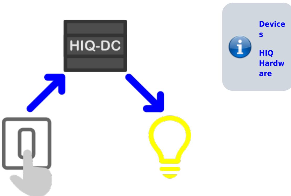
HIQ-DC are connected to each other and to **HIQ-HC** through HIQ-IEX2 control bus. Advanced functions (appliance scheduler, scenes, ...) are implemented on other HIQ-DC or on connected HIQ-HC. Due to hi-speed and reliable **HIQ-IEX2** bus communication, those functions are quick and reliable.
