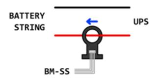
Optional, limited by the length of the included cables For proper mounting, an arrow is marked on the sensor to indicate the direction of the electric current
